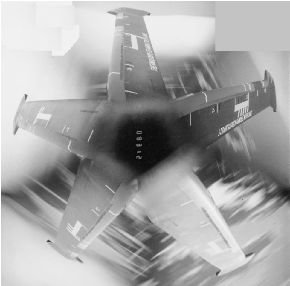
Fig. 7.28 Typical photograph of blade in flight (hingeless Westland 'Scout', 53.5 m/s, \psi = 290^\circ )
