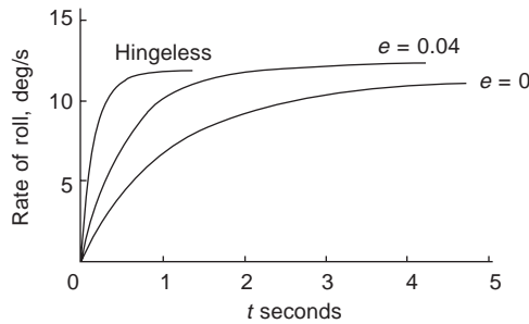
Fig. 5.25 Rate of roll in response to sudden application of lateral control
