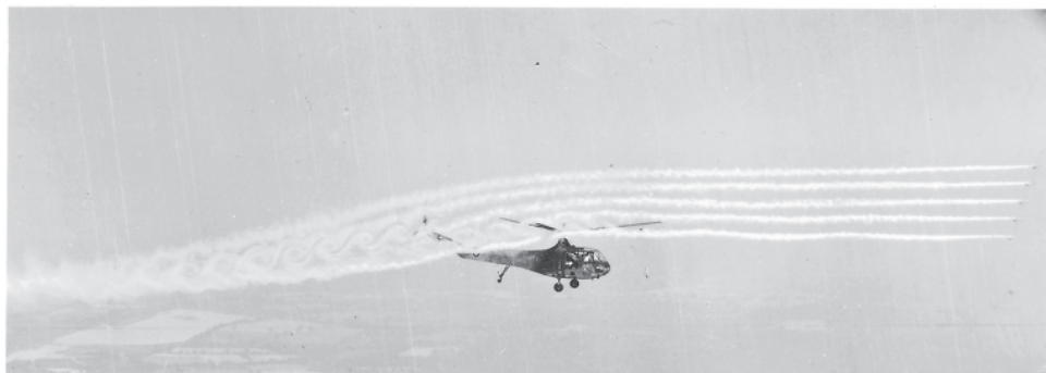
Fig. 3.8 Flow pattern as revealed by smoke filaments in forward flight. Speed 53 mph. Plane of smoke filaments 0.4R to starboard
