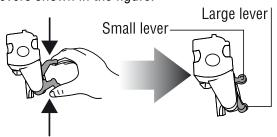
7. Once inserted, make sure the two red buttons have snapped out.
