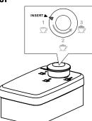
the "INSERT" position (see figure) and pull it off upwards.
