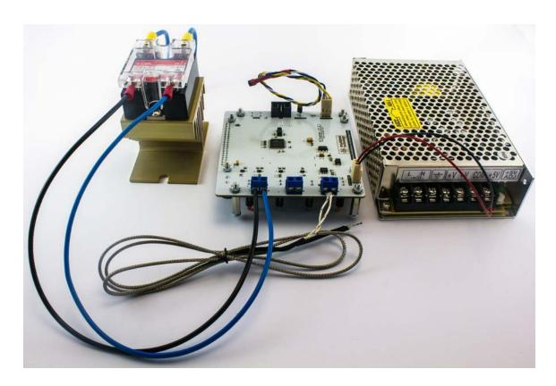
In the kit you will find the right female connectors which mates with the onboard males. Please note that it is a polarized connection and, even if the board is protected against inverted power, you should check the polarity of your power supply and connect it accordingly.
