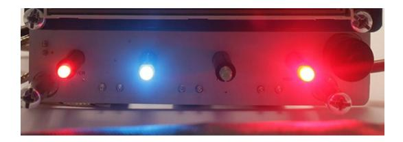
Please note that all the leds has been polarized to have mostly the same light intensity except for the SSR HEATER which is a little bit brighter (electricity is flowing, heat is generated)
