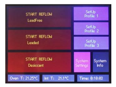
From here you can check the oven's temperature as read from the thermocouple, the onboard temperature sensor readings and how much time passed since the board was powered.
