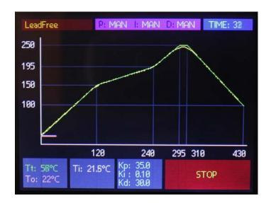
Reflow page is mostly occupied by the time/temperature graph in which you can confront the target ideal temperature (green) and the measured temperature from the thermocouple (red).
