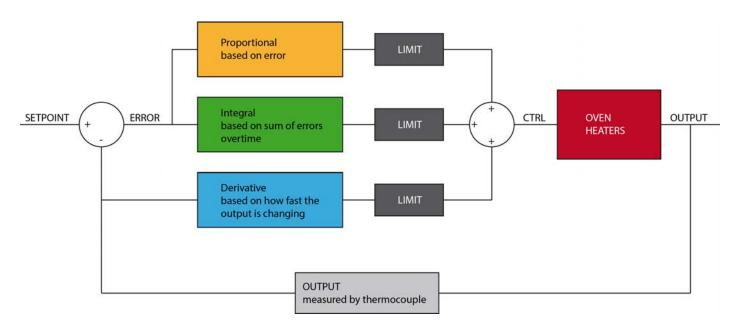
Since PID variables may become very large, they are also limited to a maximum value of  $\pm$ -999. Keep in mind anyway that a PID value of 400 (sum of P,I,D) will turn on the oven constantly, so your values should remain much lower than maximum at any time.
