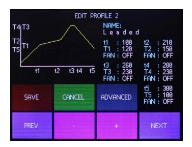
Each profile has five time nodes arranged in this way (t0 is the moment in which the reflow profile is started, for t0 temperature is automatically read from the oven):
