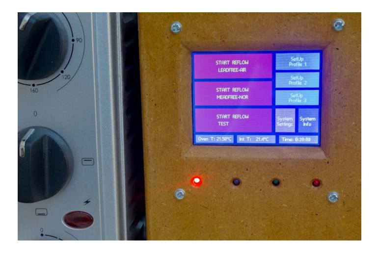
X-toaster has been designed to nicely fit in an enclosure with an inner width of about 100mm and it comes with a set of mounting spacer bolts which allows the LCD and the LEDs to sit at the right height when mounted on a front panel.
