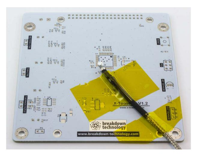
If you decided to use an unmodded oven the only way to put the thermocouple inside the oven is through the main door.
