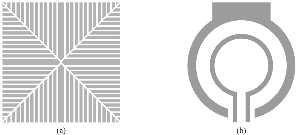
Figure 6.6 (a) A patterned shield is employed to prevent electrical fields from penetrating the substrate while preventing eddy current (closed loops) flow over a large area. (b) A co-planar ground shield improves the quality factor of the ring inductor by intercepting a fraction of the fringing fields from reaching the lossy ground.
