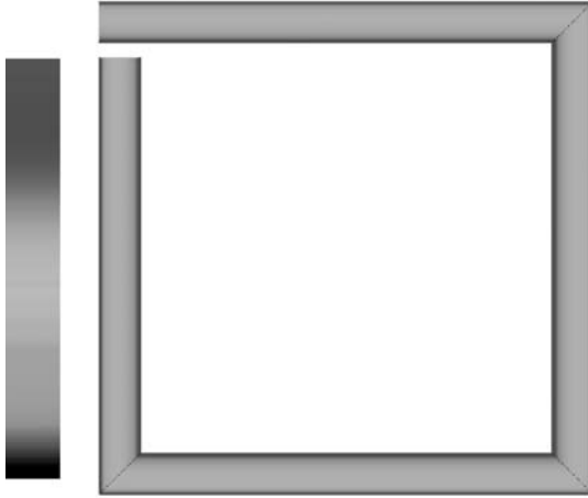
Figure 6.3 Current constriction in a square ring inductor.
