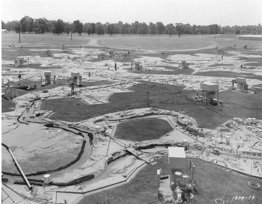
Figure 8.6 Model of the Mississippi River. Photo is courtesy of U.S. Army Corps of Engineers Waterways Experiment Station, Vicksburg, Mississippi. Reprinted with permission. Note the scale indicated by the people in several locations in the photo.
