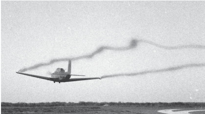
Figure 1.2 Aircraft wingtip vortices. Smoke is introduced at the wingtip to mark the vortex cores. Photograph by W. L. Oberkampf.
