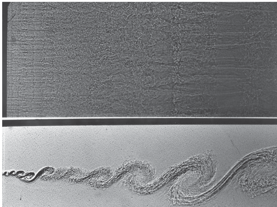
Figure 26.28 Growth of a free-shear layer between streams with different speeds. The lower portion of the photo is a side view; a plan view is reflected in a mirror in the upper portion. Large coherent eddies continue to grow for all downstream distances. Reprinted with permission from Brown and Roshko (1974).
