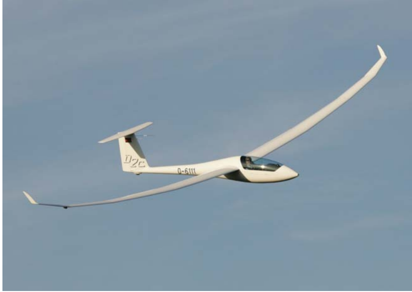
Figure 19.14 Schempp-Hirth Discus 2C is a 18-m sailplane with winglets using PSU 94-097 airfoils. Photograph courtesy of Professor M. Maughmer, Pennsylvania State University and Schempp-Hirth Flugzeugbau GmbH, Kirchheim/Tech, Germany.
