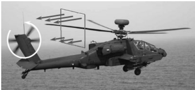
Figure 6.15 Incident flow over tail rotor (Courtesy US Navy)
