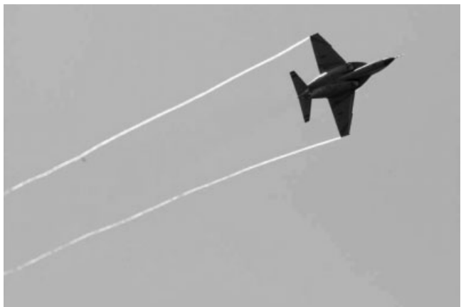
Figure 1.18 Tip vortices generated by a fixed-wing aircraft
