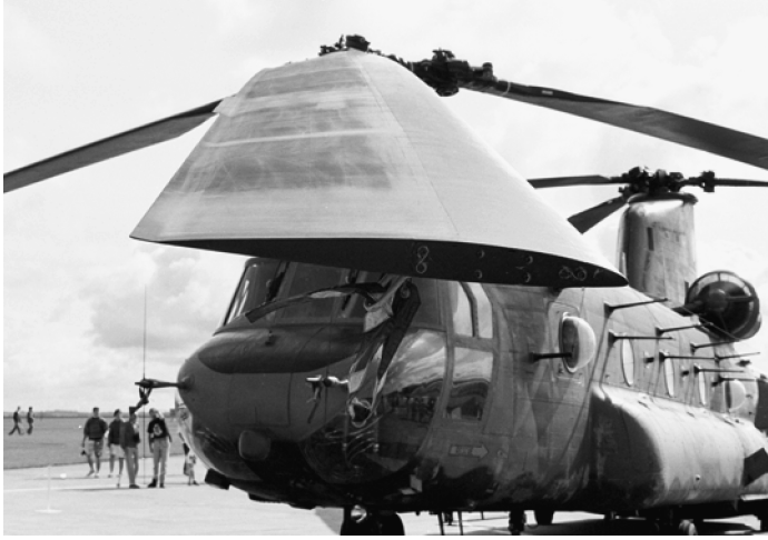
Figure 3.7 View along Boeing Chinook main rotor blade showing twist
