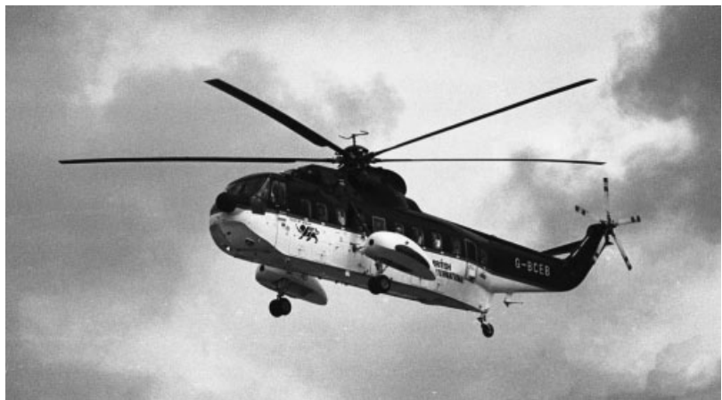
Figure 6.6 Rectangular blade planform of S61NM helicopter
