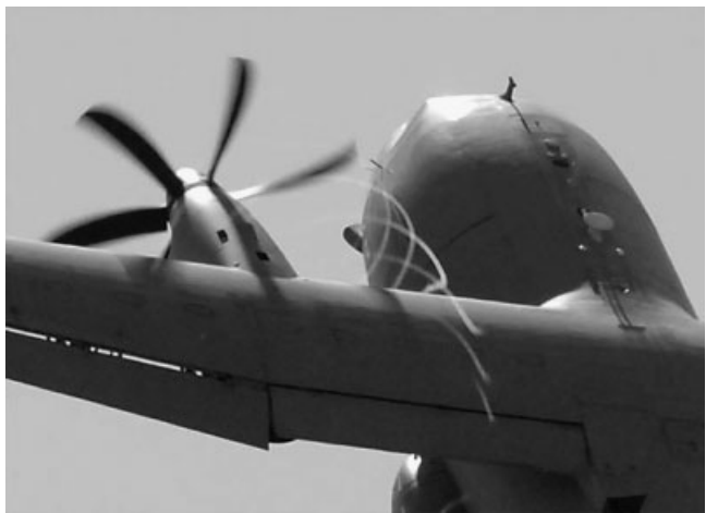
Figure 1.19 Propeller tip vortices
