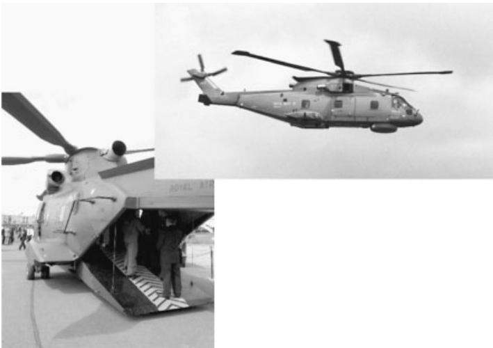
Figure 6.33 Shapes of Merlin fuselage both standard and that fitted with a rear loading ramp
