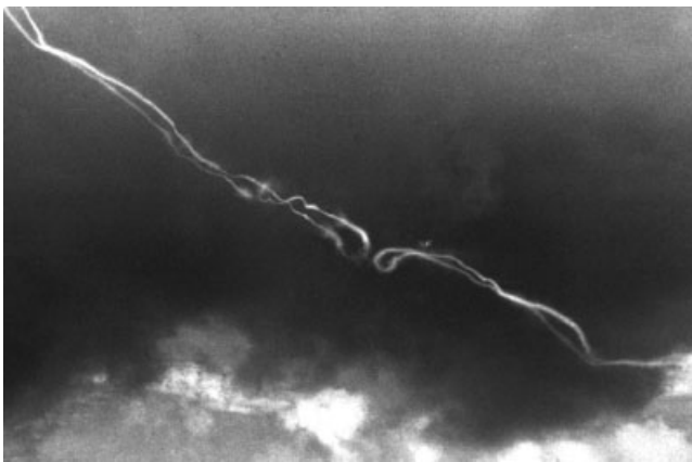
Figure 1.21 Wing tip vortices (BAE Hawk 200)
