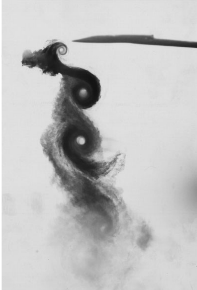
Figure 2.26 Real rotor wake
