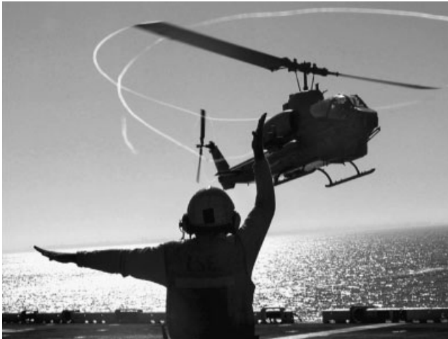
Figure 1.20 Rotor blade tip vortex trajectories (AH-1W) (Courtesy Safety Centre US Navy)
