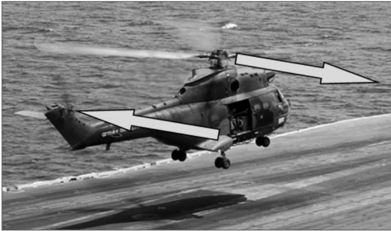
Figure 6.13 Puma hovering showing tail rotor thrust direction and opposing main rotor side force (Courtesy US Navy)
