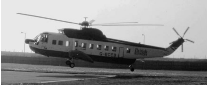
Figure 4.5 Sikorsky S61NM helicopter approaching touchdown (coned rotor)
