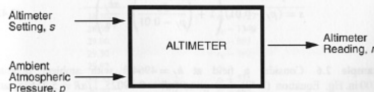
Figure 2.6 Input and output variables for the altimeter.
