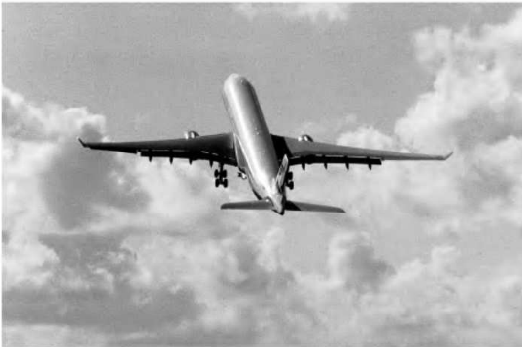
Fig 7B Climbing An Airbus A-330 using flaps to demonstrate its steep climb capability.
