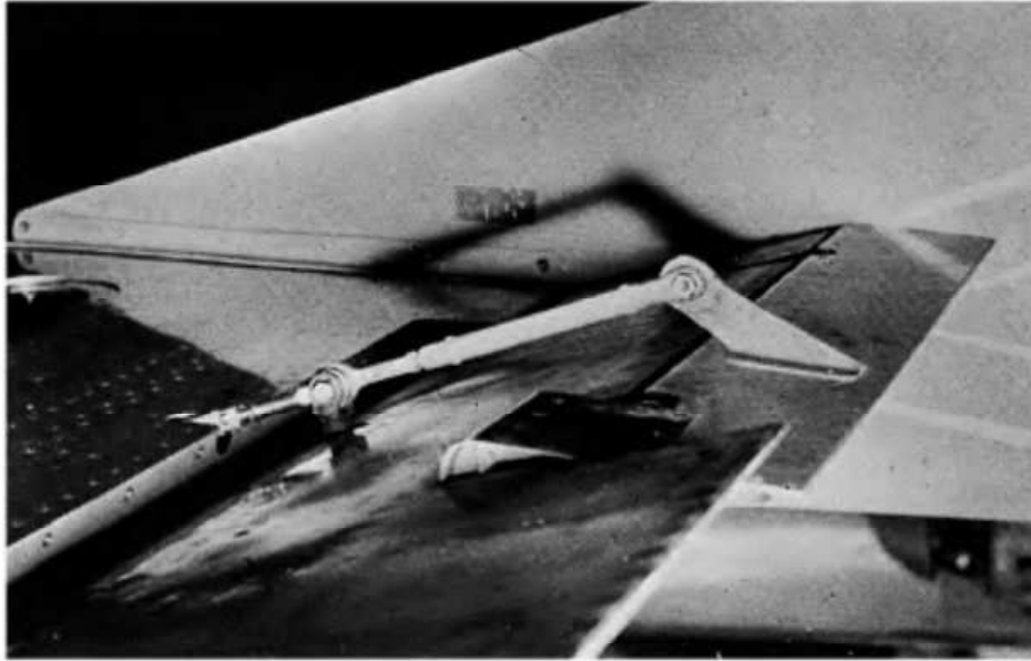
Fig 9I Tab control mechanism (By courtesy of Piaggio, Genoa, Italy)
