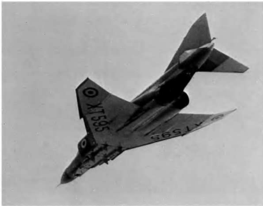
Fig 11E Saw-tooth or dog-tooth (By courtesy of McDonnell Douglas Corporation, USA) The Phantom (RAF version), showing clearly the dog-tooth on the leading edge; the outer wings have 12^\circ dihedral; there are blown leading and trailing edge flaps; the slab tail has 15^\circ anhedral and a fixed slot; the rudder is inter-connected with the ailerons at low speeds.
