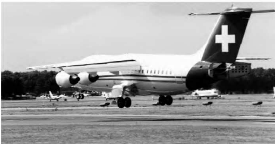
Fig 6J Landing A BAe 146 about to touch down, Fowler flaps extended and rear air-brake doors open.
