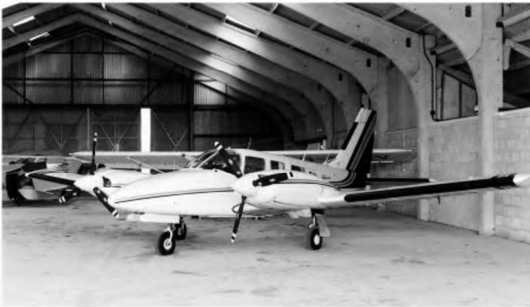
Fig 4E Piston engine and propeller The piston engine and propeller is still the most common arrangement for light general aviation aircraft.
