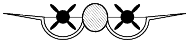
Fig 6.8 The idea of the ‘Custer’ channel wing The engines – with pusher propellers – were suspended in the channels with the ailerons just outboard of the channels.
