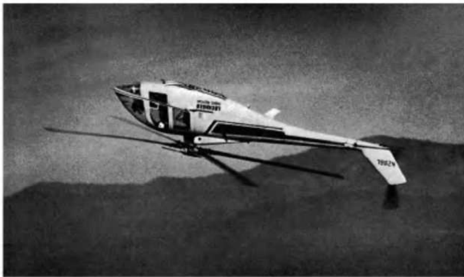
Fig 8D Manoeuvres (By courtesy of the Lockheed Aircraft Corporation, USA) A rigid-rotor helicopter performing aerobatic manoeuvres.
