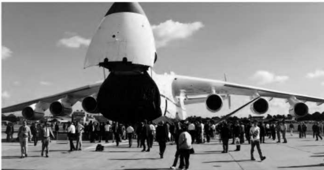
Fig 1A Weight and thrust The massive Antonov An-255 Mriya, with a maximum take-off weight of 5886 kN (600 tonnes). The six Soloviev D-18T turbopfans deliver a total maximum thrust of 1377 kN.
