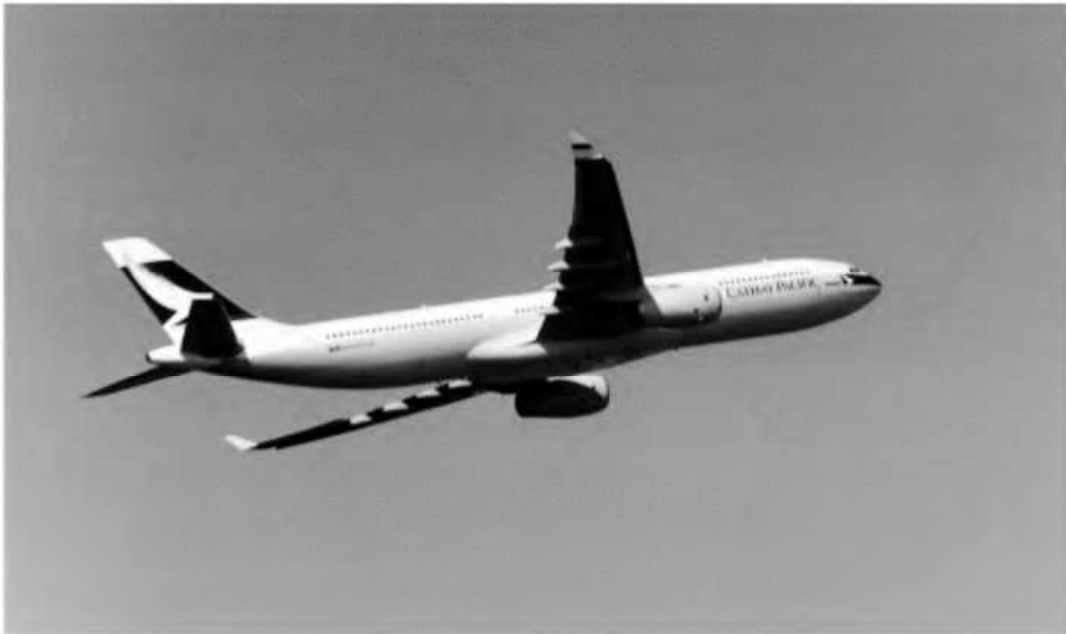
Fig 9C Sweepback An Airbus A330 showing the sweepback of the wings.
