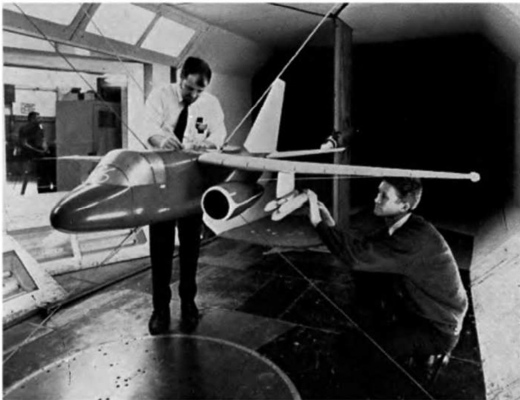
Fig 2G Model in wind tunnel (By courtesy of the Lockheed Aircraft Corporation, USA) Model being prepared for flutter tests in wind tunnel
