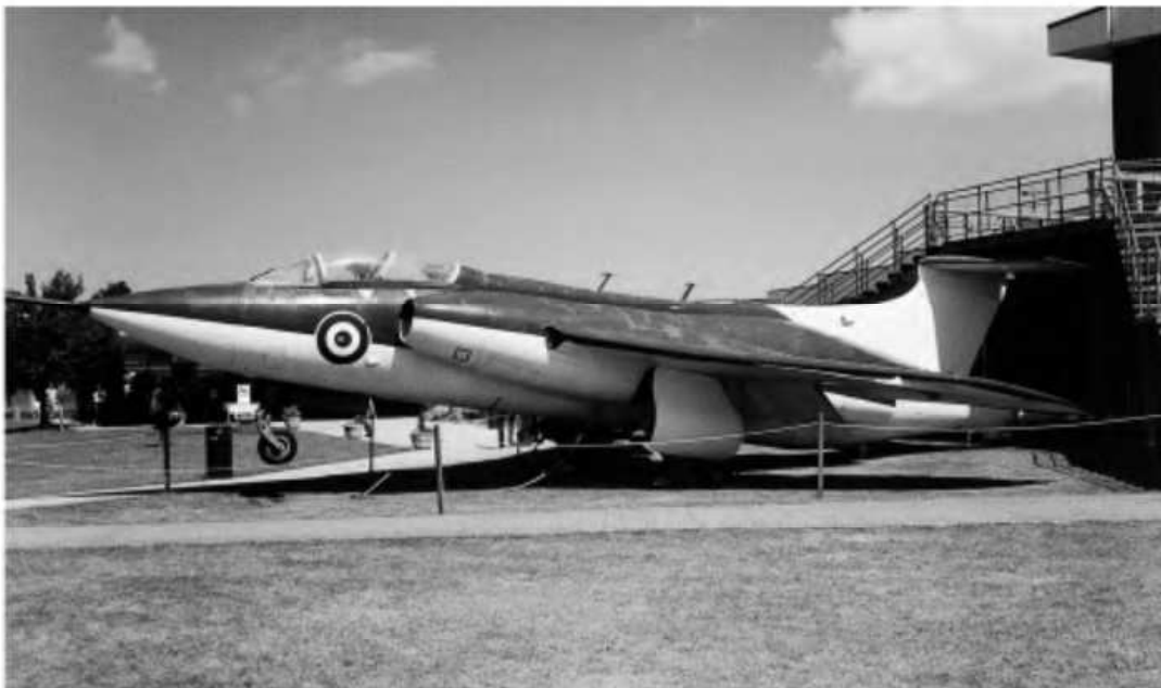
Fig 11C Transonic area rule The transonic British Aerospace Buccaneer which finally saw action in the Gulf War shortly before retirement. The bulge in the rear fuselage is for purposes of area rule.
