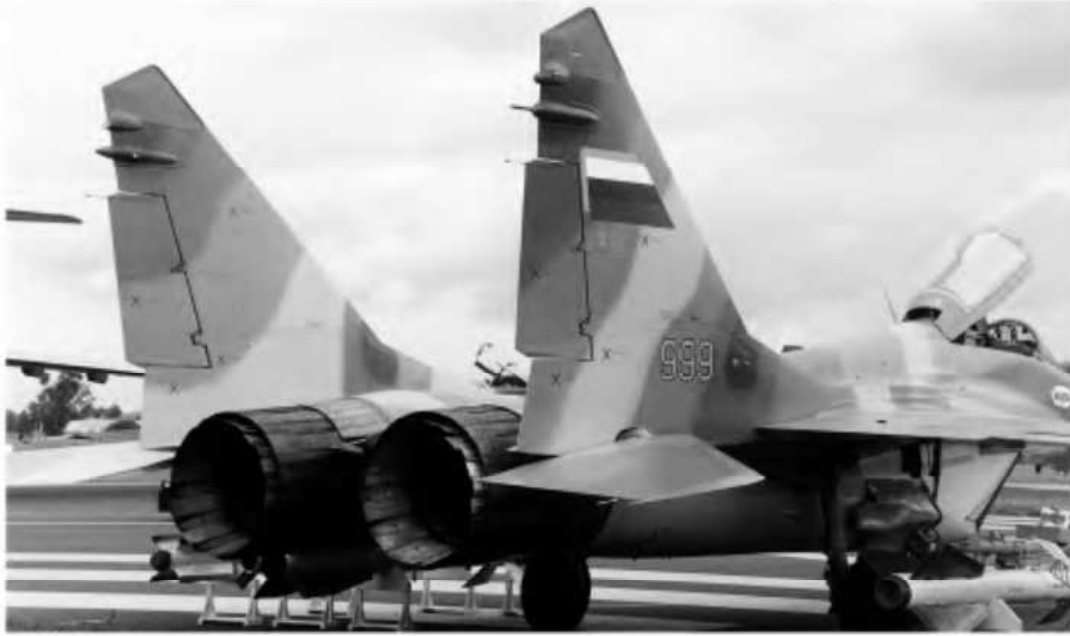
Fig 4A Turbojet propulsion The hot end of a MiG-29. Two Tumansky R-33D low-bypass turbojet engines, each producing 81.4 kN thrust (with reheat). Note the complex variable area outlet nozzles.
