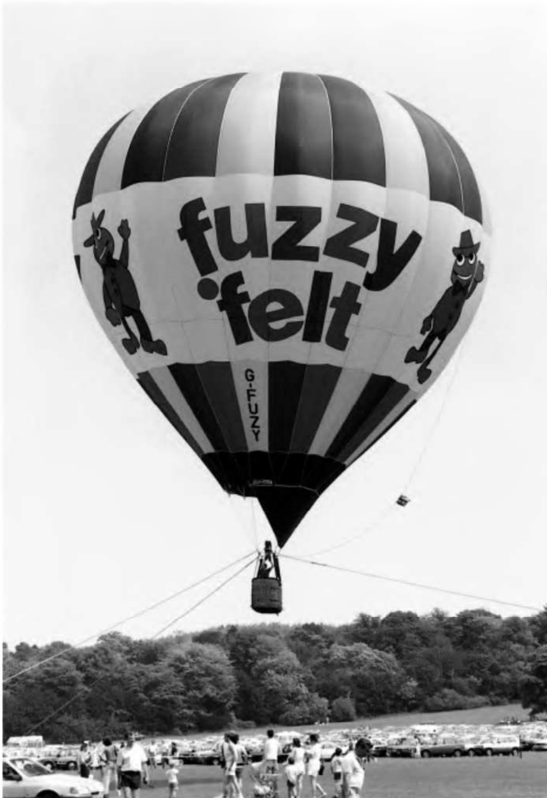
Fig 6H VTOL – another way After a century of neglect, the hot-air balloon has made a major comeback. This one is tethered and is being used for pilot training. The wicker basket provides good impact absorption on landing.
