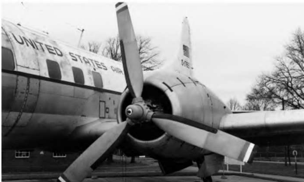
Fig 4J Constant-speed propeller A classic constant-speed propeller design. The hydraulically-actuated speed control unit is housed in the small domed unit on the front of the hub.
