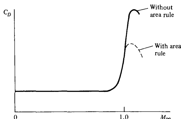
Figure 11.18 The drag-rise properties of area-ruled and non-area-ruled aircraft (schematic only).
