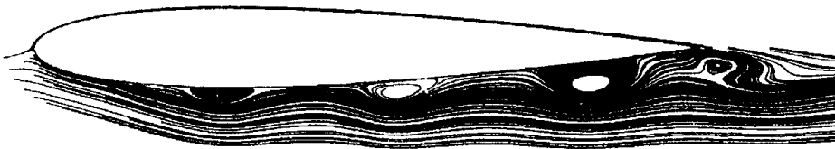
Figure 20.14 Streamline pattern over the bottom of an NACA 0012 airfoil, over which a series of jets is distributed which are alternatively blowing or sucking mass into or out of the flow, with the overall net mass injected into the flow being zero—a zero-mass jet array. (Source: Hassan and JanakiRam, Reference 91.)
