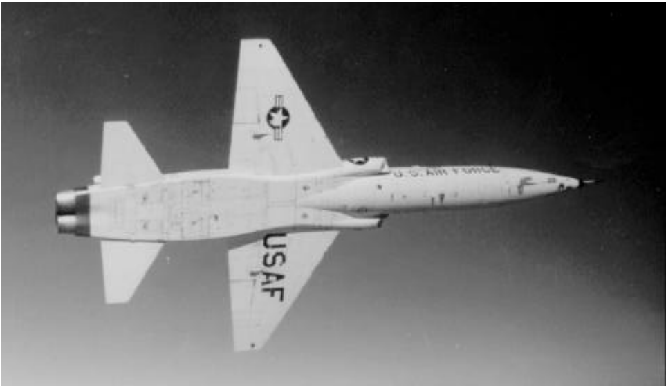
Figure 4.33 Area Ruling of the T-38 Fuselage (Brandt collection)
