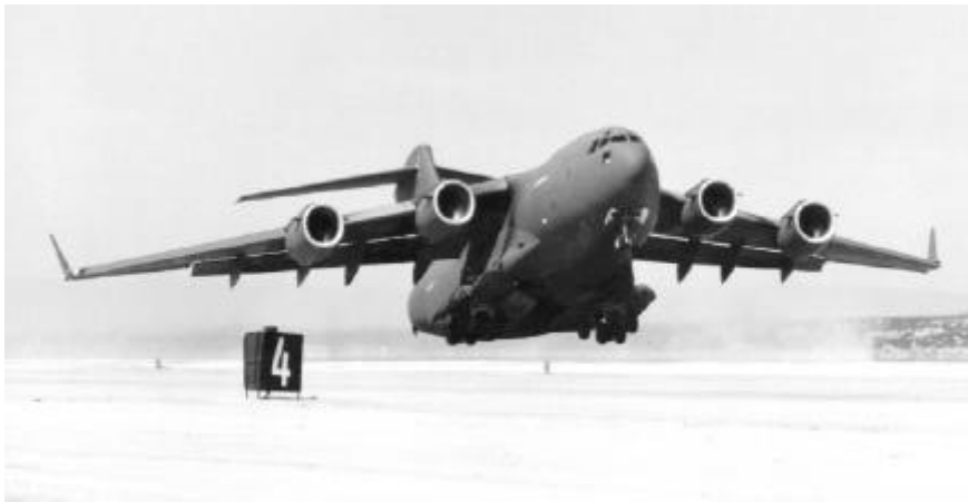
(b) Winglets on a C-17 (USAF Photo)
