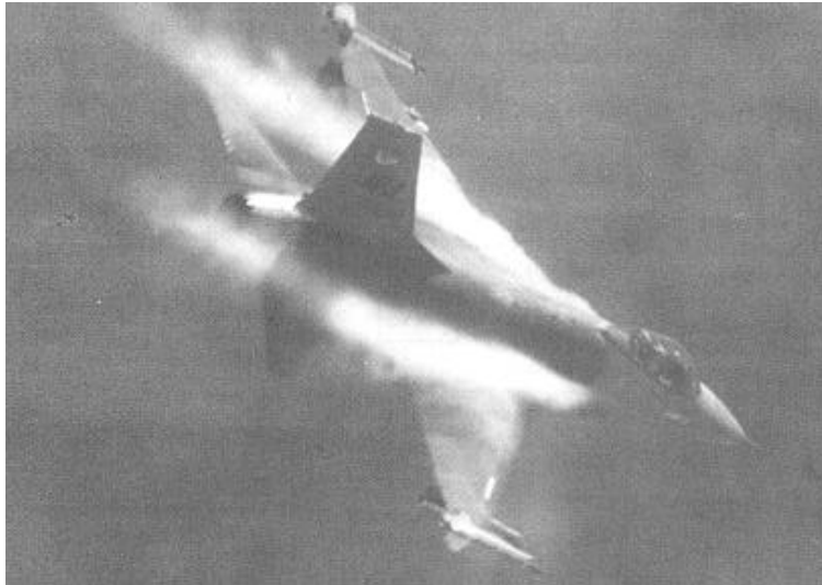
Figure 9.14 The Complex Flowfield over a Wing with Leading-Edge Vortices (Courtesy Lockheed-Martin)
